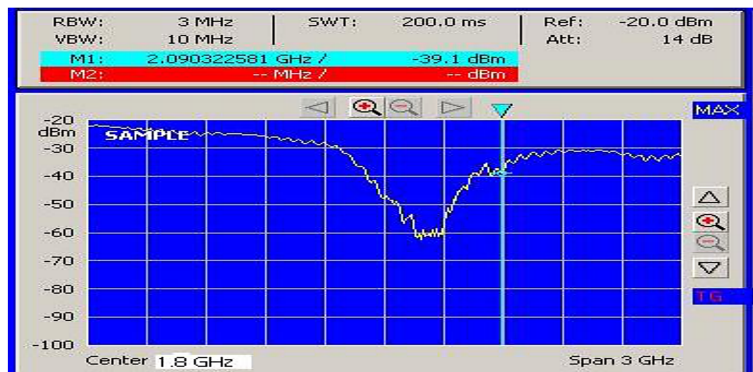
Figure 3(b): measured response of microstrip optimum band-stop filter
