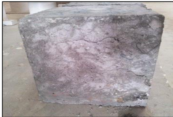
Figure 22. Cubes after failure under Compression load
